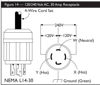
This receptacle powers 120/240 Volt AC, 60 Hz, single phase loads requiring up to 3,600 watts of power at 30 Amps for 120 Volts; 7,200 watts of power (7.2 kW) at 30 Amps for 240 Volts. The outlet is protected by a 30 Amp push-to-reset circuit breaker.
